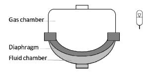
It consists of two steel shells (hemispheres) and a flexible synthetic diaphragm. The diaphragm is used to separate the gas and the fluid sections. The diaphragm is typically made of Buna-N, Viton, Butyl, or Hydrin. Where contamination is a serious problem, a vertical mount is preferred. It is fast acting and does not exhibit hysteresis. It reacts quickly to changes in the system pressure. The compression ratio is about 8.
