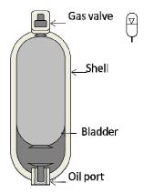
It consists of a pressure vessel (shell) and an elastomeric bladder (bag). The bladder divides the shell into a fluid chamber on the system side and a gas chamber inside the bladder. The gas chamber is pre-charged. Materials for the bladder: Buna-N (Standard material), chloroprene, nitrile, Viton, Butyl, and Hydrin. Bladder accumulators are fast acting and do not exhibit hysteresis. The compression ratio for bladder accumulators is limited to 4.
